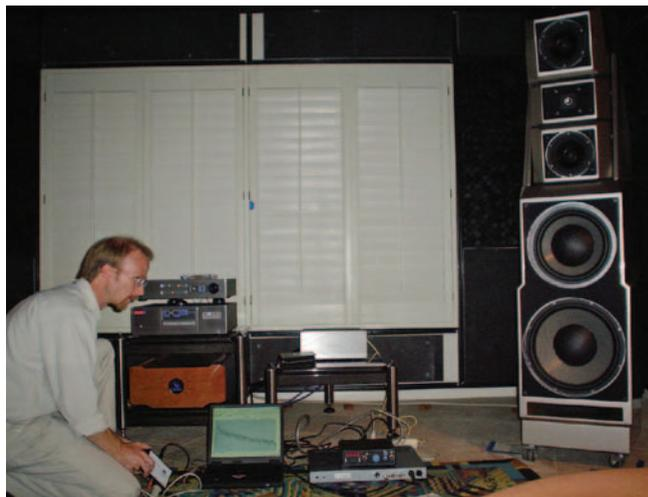
**Varney uses tools such as a sound pressure level (SPL) meter, real-time analyzer (RTA), music articulation test tone (MATT) and time energy frequency (TEF) equipment to position speakers.**
