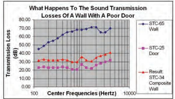
Figure 5: Note that the partition is heavily affected by the weakest part of the system (see Figure 5), which is typically a door or window. Note also how a small leak affects the assembly’s performance. A 1 percent leak area can never exceed STC 20, no matter how good the partition’s potential.
