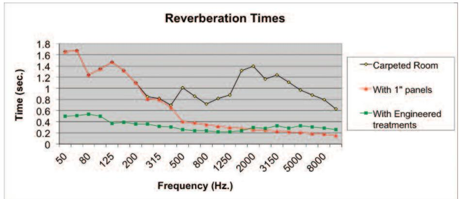
Fig 3. Actual reverberation test data of a typical home theatre without additional acoustic treatments, with optimized typical treatments, and with engineered treatments. More commonly, the red curve dips lower beginning at around 500 Hz.
