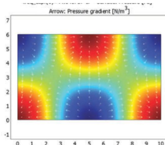
Graph 6. Measurement snapshot of a room mode. This can represent a floor or elevation plan view. Shown are strong fundamental modes in the corners and middle of the room.
