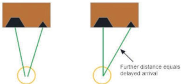
Graph 3. Indicating how if the loudspeaker is not oriented (tilted/angled) properly to the listener, time arrivals are distorted, causing frequency response anomalies.
