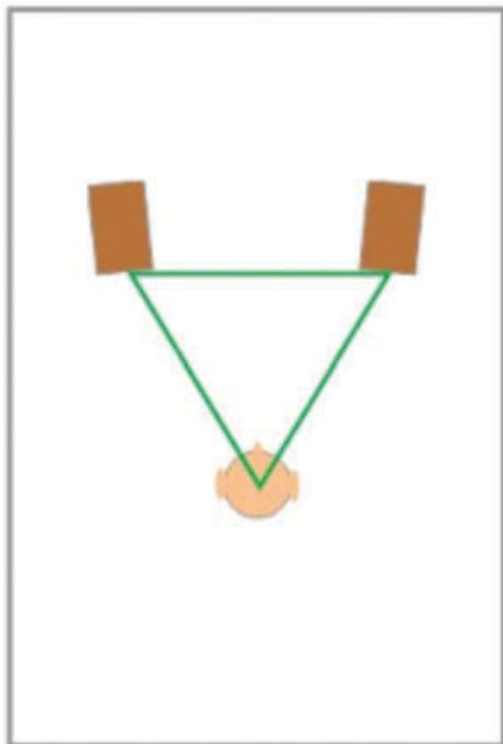
Graph 2. Stereo foundation showing equidistant triangle. This is a good way to start setting up the best soundstage. Loudspeaker toe-in angle will also affect soundstage and timbre.
